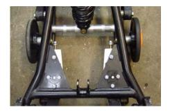
4. Using the supplied ¼"x ¾" flat socket head cap screws and nylon locking nuts bolt a strap adjuster to the bottom of each plate. Then thread your limiter strap thru the strap adjuster bolt and attach the strap to the aluminum strap adjuster block and front arm plate using the supplied 1/4" x 1" cap screw, washer, and nylon locking nut. The limiter straps have three holes in them. Use the middle hole in the strap to attach to the
