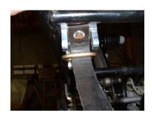
5. Push the limiter strap up against the aluminum adjuster block and slide the supplied 1/4"X 2.75" grade 8 hex head cap screw thru the cross holes. Position this bolt so the nylon locking nuts are towards the inside of the suspension as shown. Use the 1/4" flat washer and nylon locking nut to secure the bolt. Note – only snug down the nylon locking nut to keep the cross bolt from rattling. Don't over tighten the bolt as it could bend the strap adjuster side pieces.
